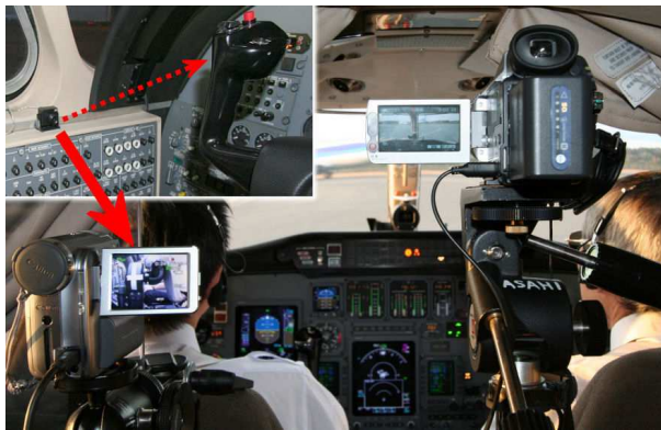
Fig. 1: The control command is recorded using a white cross marker on the column (left), the visual cues are recorded with the camera on the right.
